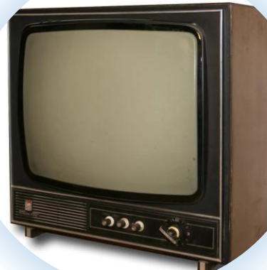
BLACK&WHITE TV: CRT, Scan 25 Hz, Diagonal - 45 cm.
